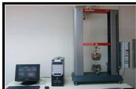
**Fig. 8.** Universal testing machine
