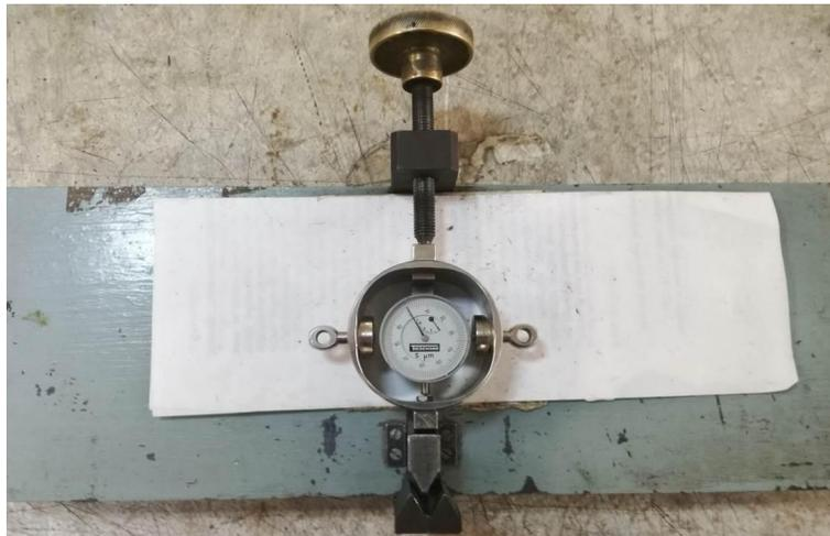
**Fig. 2. Three-point bending test machine**
