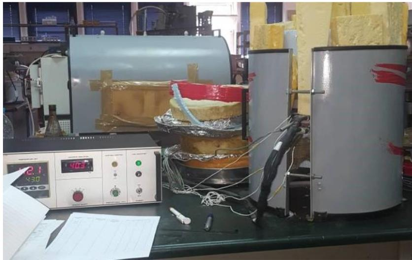
Fig. 4. Thermal conductivity measuring equipment
