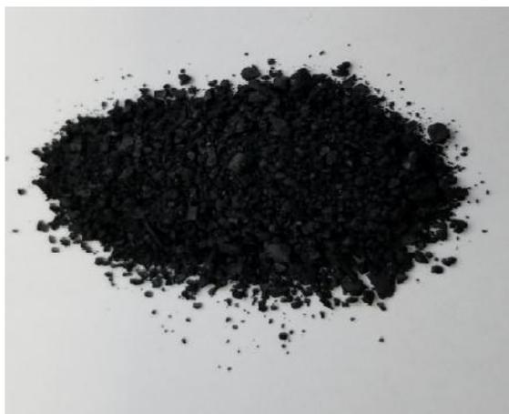
Fig. 1. Graphene oxide (GO) obtained from Hummer's method
