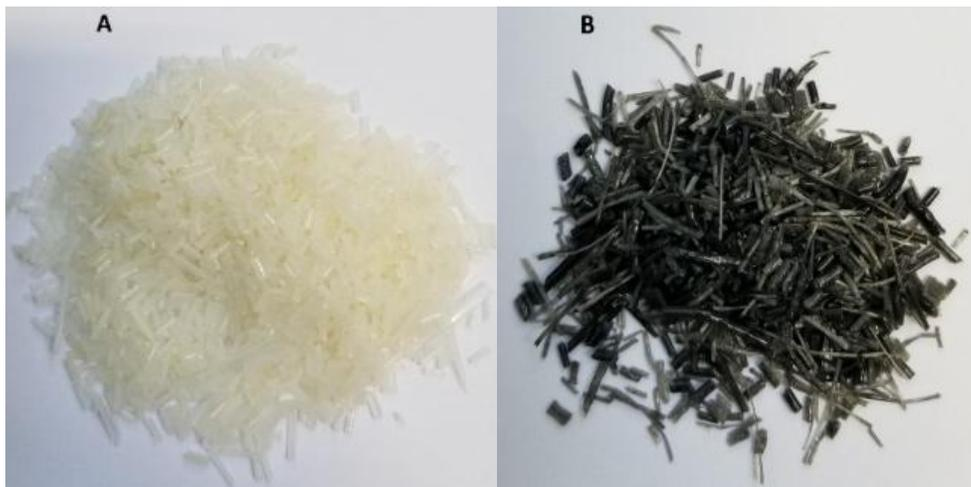
**Fig. 11. (a) Processed nylon fibers, and (b) Processed graphene-nylon fibers**
