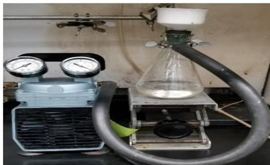
Fig. 2. Vacuum filtration set-up
