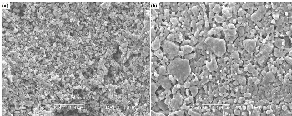
Fig. 2. SEM micrograph of the  $\text{Ca}(\text{Zn}_x\text{Ti}_{1-x})\text{O}_3$  ceramics sintered at  $1000^\circ\text{C}$  for 3 h in air; (a)  $x = 0.0$ , (b)  $x = 0.5$ ; indicating a slight change in grain sizes with increase in  $x$
