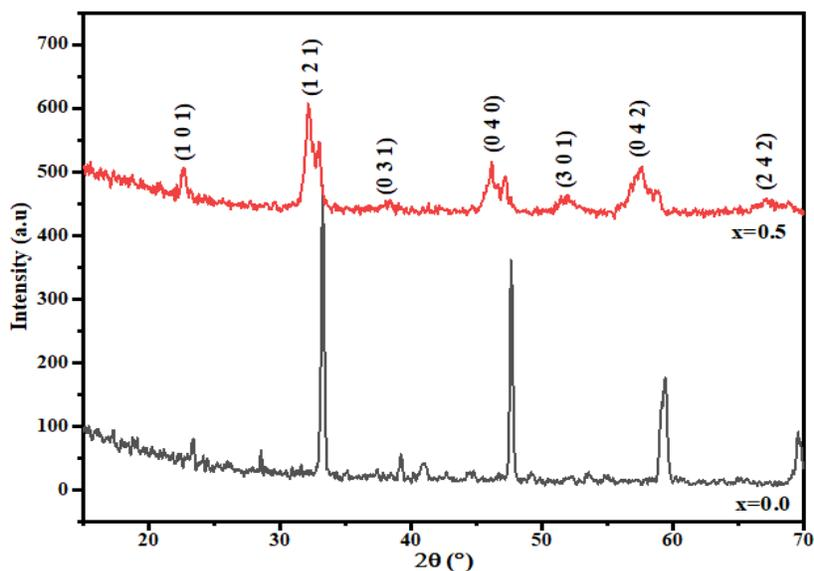
Fig. 1. XRD of  $\text{Ca}(\text{Zn}_x\text{Ti}_{1-x})\text{O}_3$  ceramics sintered at  $1000^\circ\text{C}$
