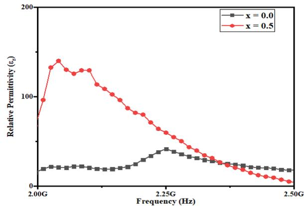
**Fig. 3. Experimental plots of the dielectric constant versus frequency of  $\text{Ca}(\text{Zn}_x\text{Ti}_{1-x})\text{O}_3$  ceramics sintered at  $1000^\circ\text{C}$  for three h in air**
