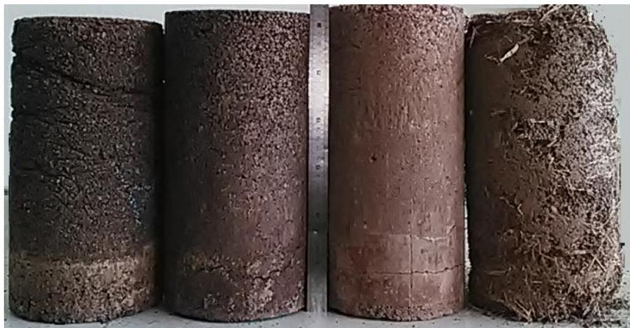
**Fig. 7. photography of samples :70%A-30%S, 65%A-30%S-5%GA, A100%, 98.5%A-1.5%P.**
